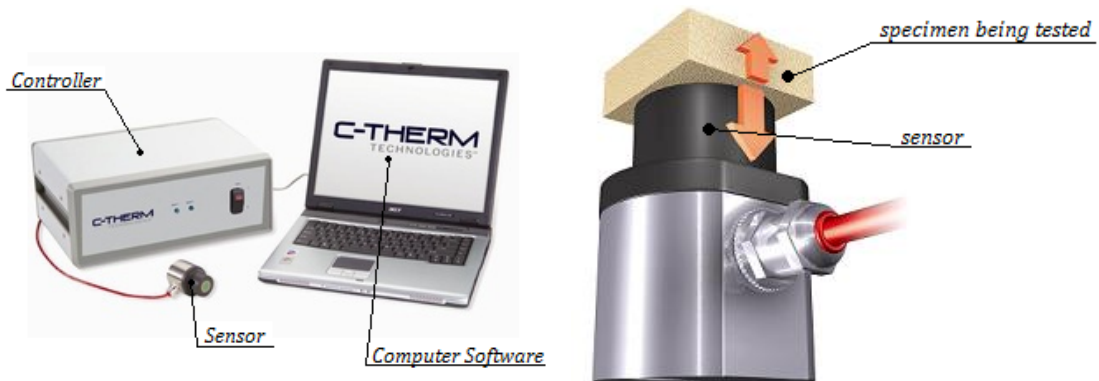
Figure 3 – C-Therm TCi thermal conductivity analyzer: (a) C-Therm TCi system; (b) Sensor in use.
