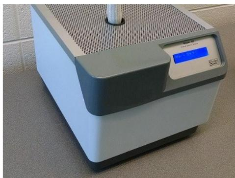
Simplex Infrared Spectral Detector for TGA
