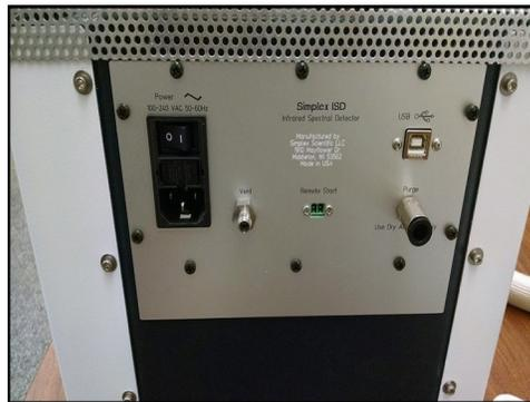
ISD back panel, Universal AC input auto switches voltage for use worldwide
