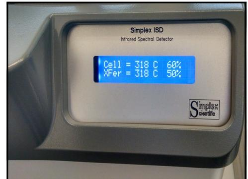
Display showing temperature of Transferline and Cell
